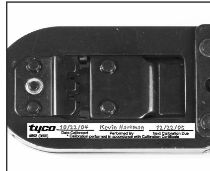
**A label conveniently located on the crimp head, which moves with the head from tool to tool, lets the operator see when calibration or inspection is due.**
